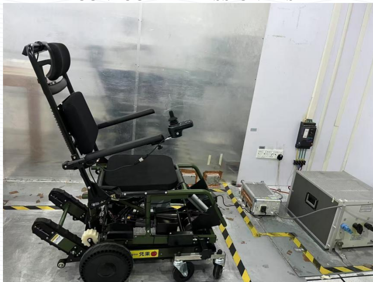
Figure 1 CONDUCTED EMISSION TEST
